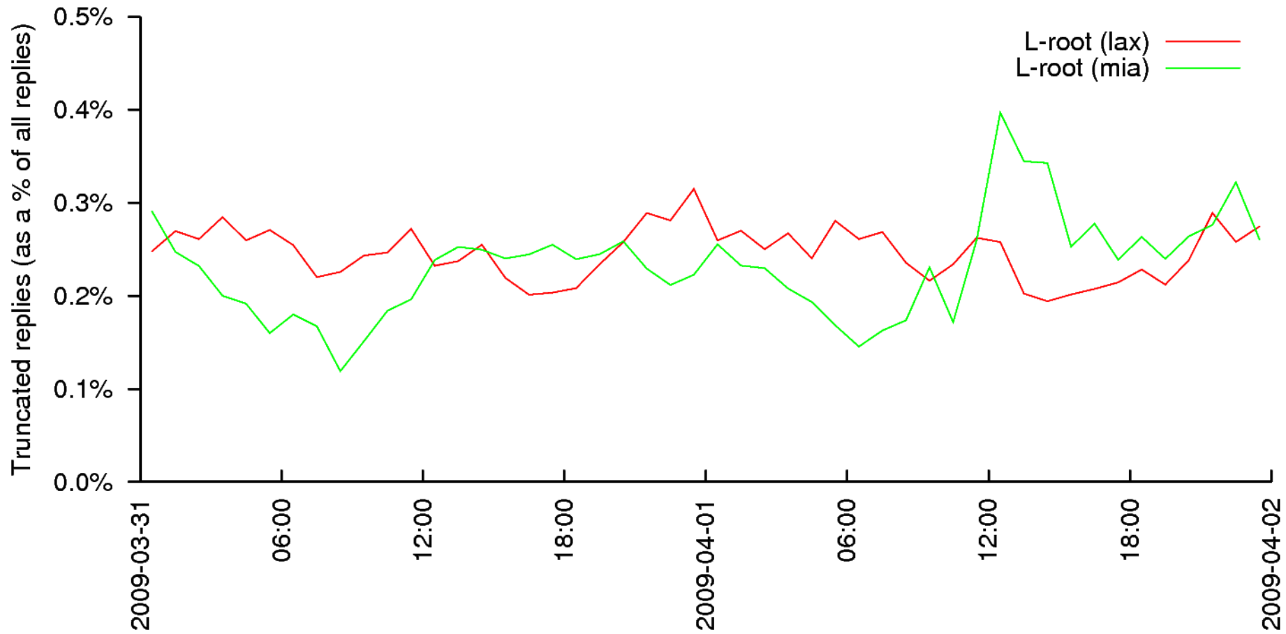
Rates of Truncated Replies from L-Root Simulation Serving Singed Root Zone (abnormal queries removed).
