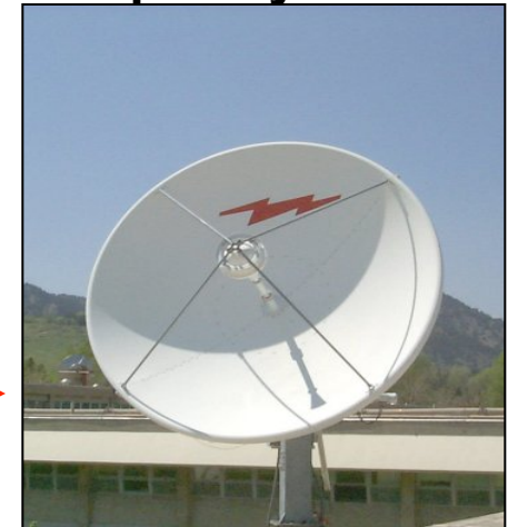
Two-way satellite time & frequency transfer
