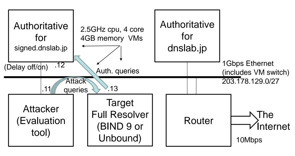
Evaluation tool sends (random).signed.dnslab.jp A queries to the target Before experiments, "dig @target signed.dnslab.jp SOA"
